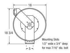
Oxy Inlet — 1/4" FPT Acet Inlet — 1/4" FPT Max. Temp.  $-200^{\circ}F$
